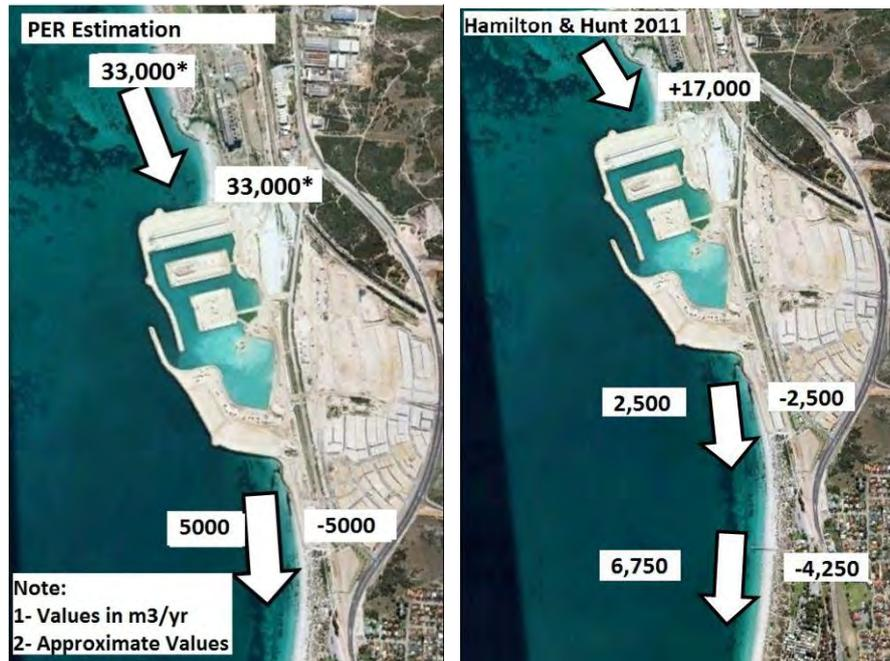
*Figure 6: Estimated net sediment movement 2005 to 2009 prior to first sand bypassing operation. (Hamilton & Hunt 2011)*
