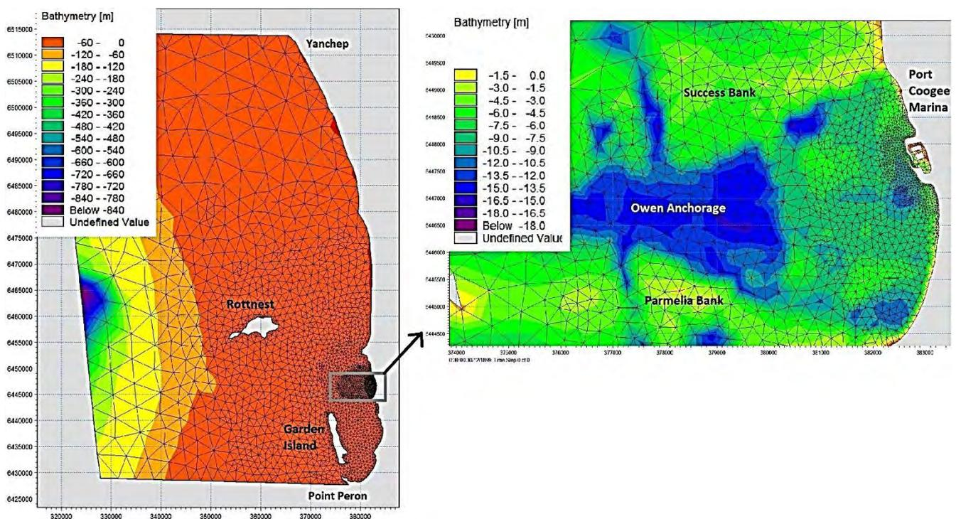
**Figure 9: Model boundary and computational grid**
